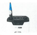
2 Connect the OAE probe to the probe socket, aligning the 'key' and 'keyway.' Screw up the knurled sleeve until finger tight.
