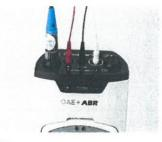
3 Plug the electrode connector leads into the appropriate sockets, following the colour coding. Push in firmly.
